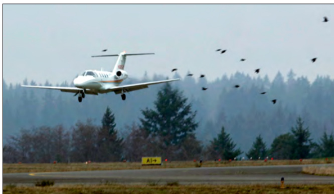
Waterfowl, gulls, and raptors represent 77 percent of reported bird strikes causing damage to aircraft in the US. Over 70 percent of all strikes occur within 500 vertical feet within the airport traffic pattern. (Photo courtesy of the Tacoma News Tribune)
